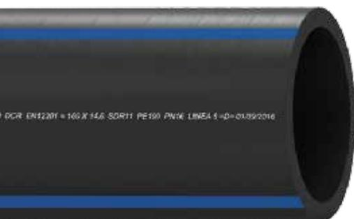
High density polyethylene pipes produced entirely of PE100 resin (MRS  $\geq 10$  MPa) highly resistant to chlorine components ( $\text{ClO}_2$ ) dissolved in the water transported, all complying with EN 12201.
