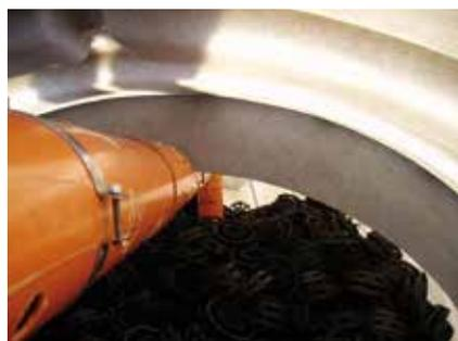
Anaerobic percolating filter.
